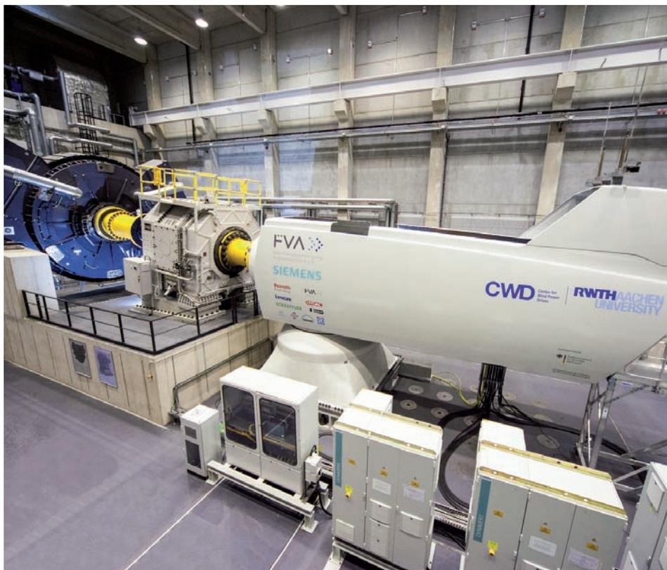
The FVA nacelle is used amongst other things to investigate electromechanical loads on the generic wind turbine generator. The aim is to develop a structurally dynamic complete model of the generator (see page 2).
